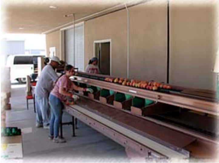
Students measure size and color of fruit on automatic fruit sorter.
